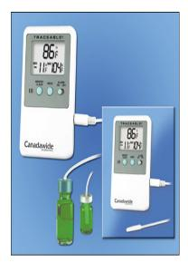
The Min/Max thermometer has a digital readout and a wire probe that is long enough to remain permanently inserted in the fridge. The probe should be attached to a water bottle or Glycol solution or inside an empty vaccine box. The digital readout should be in an easy to read location (not in the fridge). Temperatures are checked twice a day.
